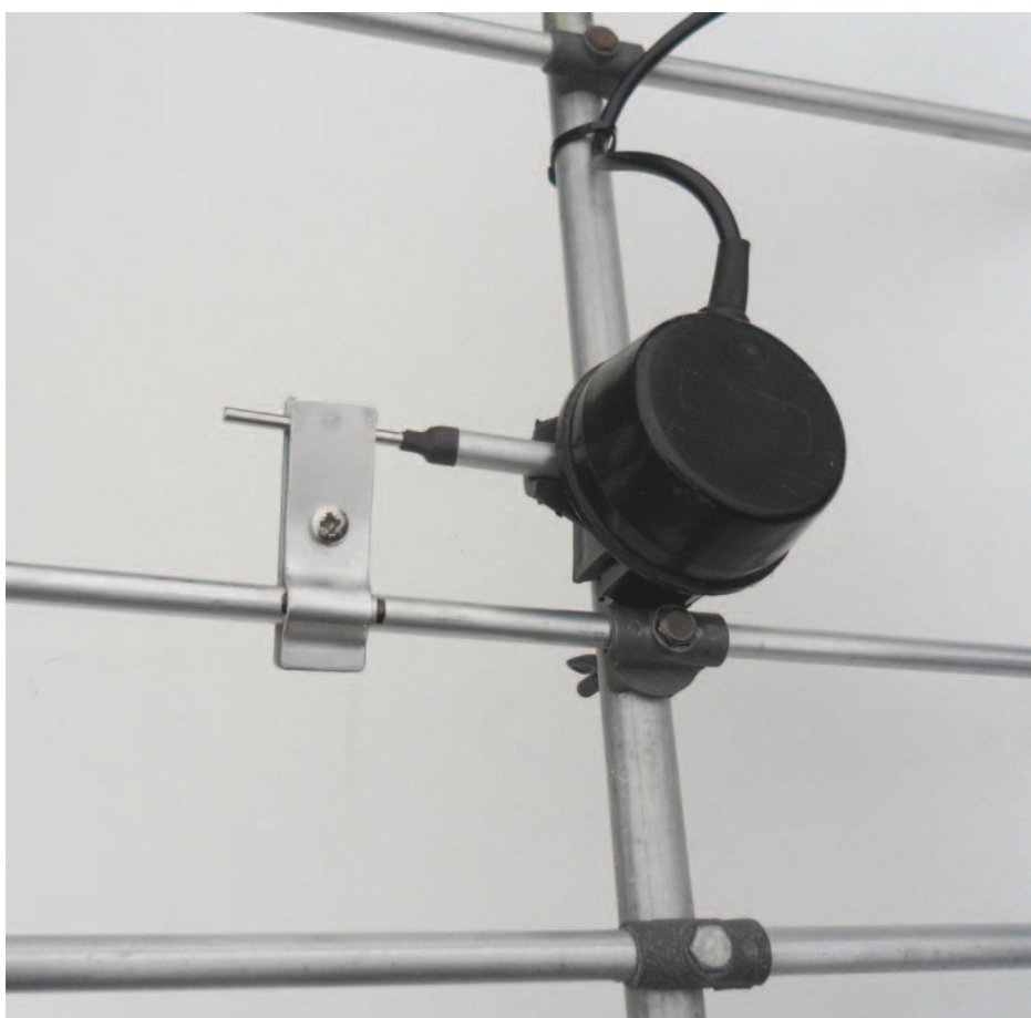
PHOTO 3: G0JMI's gamma match used on a 70cm beam.
