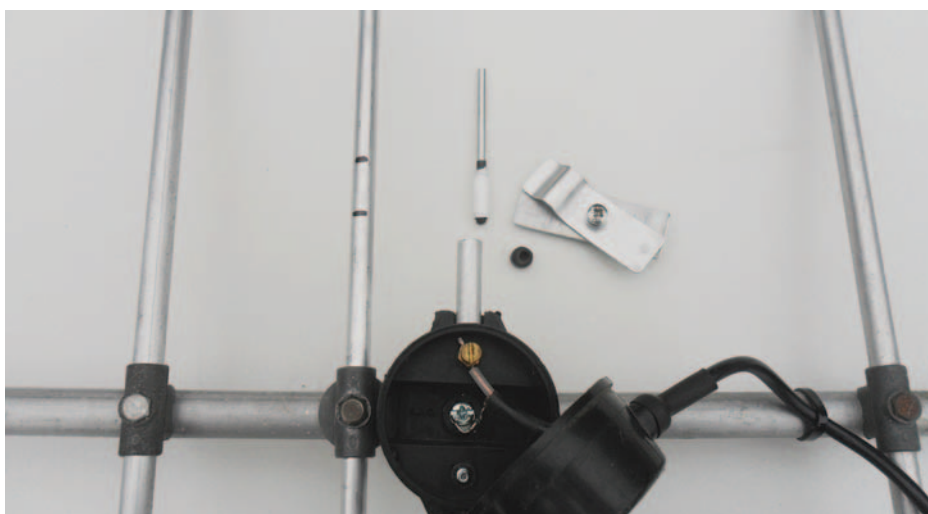
PHOTO 4: Components of the gamma match used on the 70cm beam.
