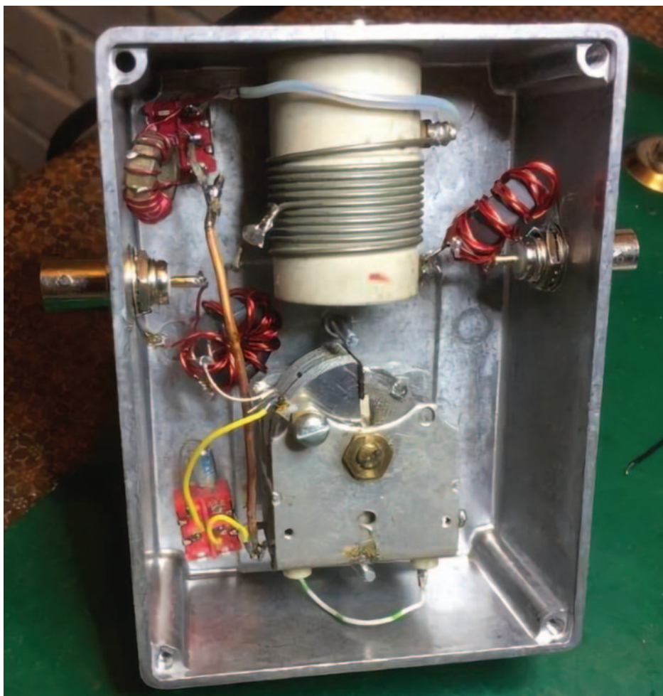
PHOTO 1: Inside one of the prototype filters. This differs from Figure 4 in that it has a switch to select between two different inductors (one on the white former, the other on a smaller toroid to the left).
