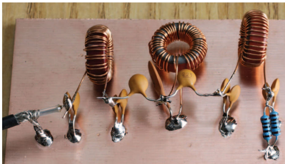
PHOTO 2: Completed prototype 160m bandpass filter.
