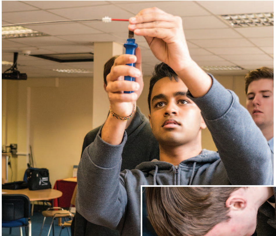
An antenna was tuned by slowly cutting it to size.
